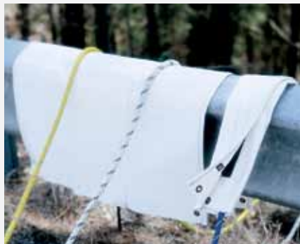
(Left) Wide Rope Pad (Right) Narrow Rope Pad with Velcro
